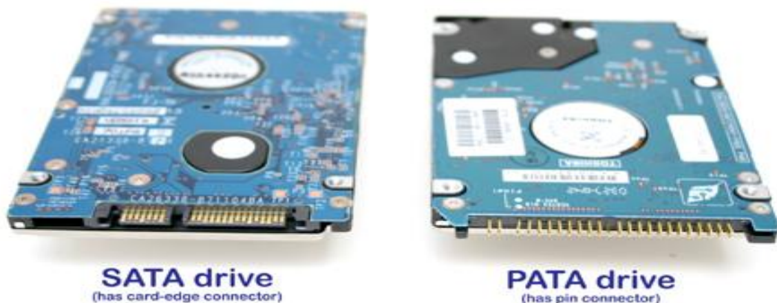
Fig. 1.4 SATA and PATA Drives
